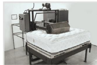
There is a standard industry test for the materials used in a mattress. It is called the rollator test and consists of a 6-sided roller weighing 230 pounds that rolled back and forth over a mattress 200,000 times. This test simulates the amount of wear that will occur as the mattress is slept on.
